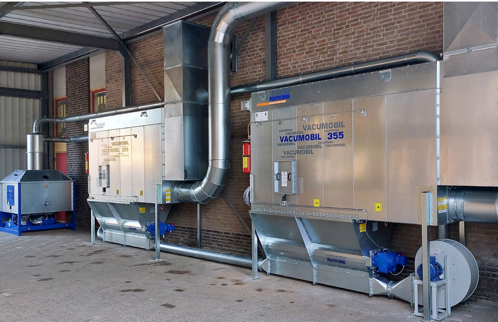
Double dust extractor JZ 355-EU with clean-air transport fan, feeding a briquetting machine for waste disposal.
